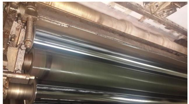
Pic: Paper Printing machine with a thin layer of water surrounding the rolling cylinder in Printing industry
