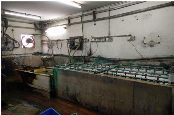
Pic: Electroplating bath for nickel and chromium surface coating in Electroplating industry
