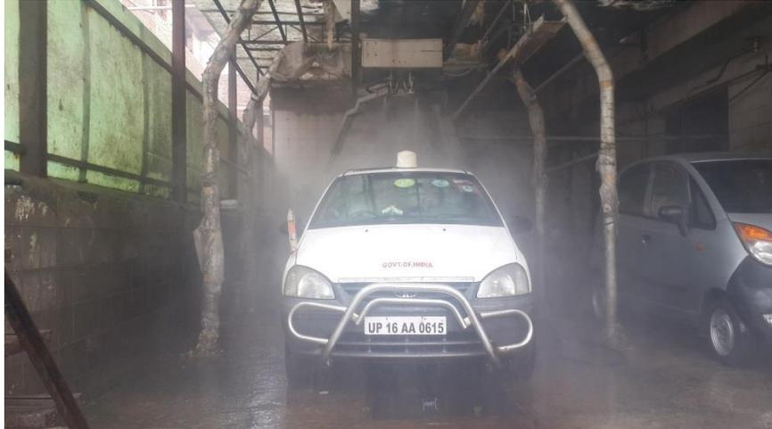
Pic: Passenger car service station with automated water wash system
