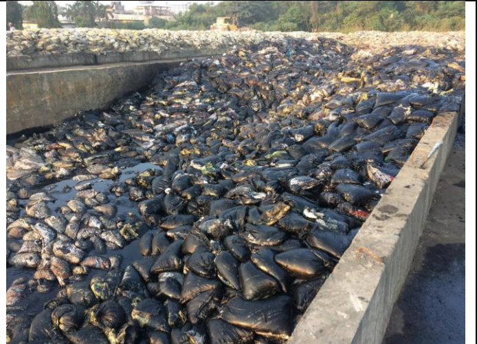
Sludge after mechanical dewatering
